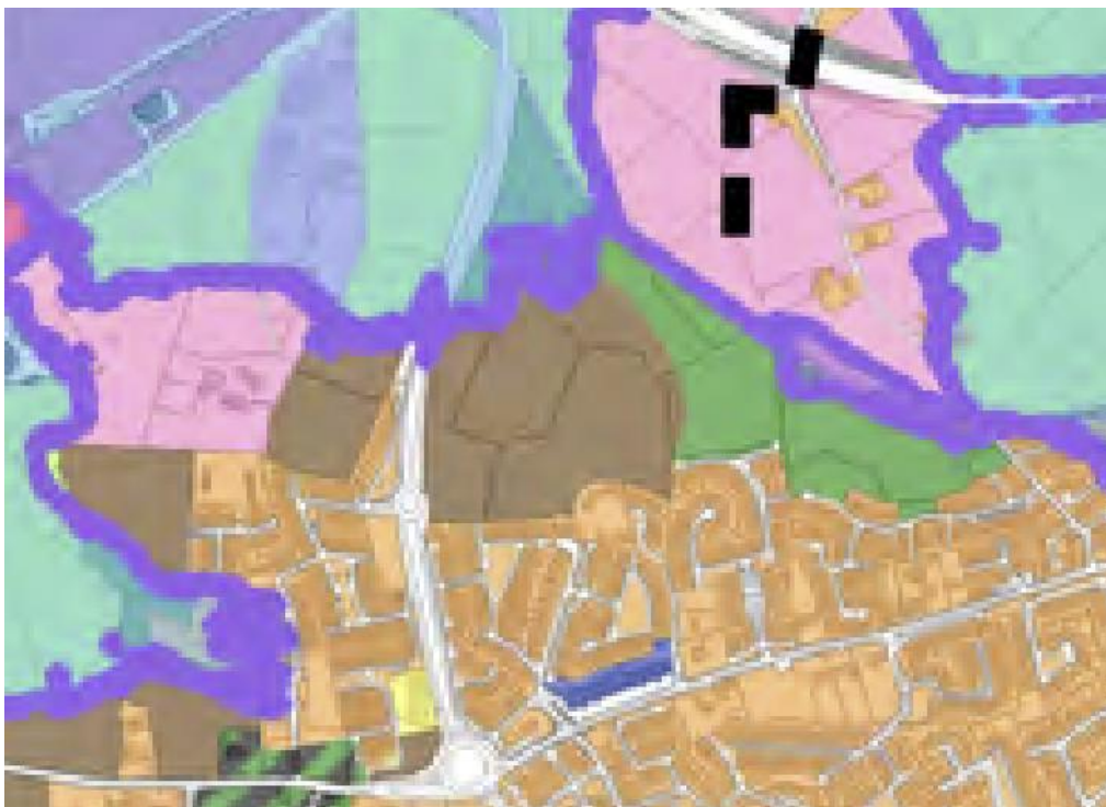
Figure 3. Flood Zones (purple) impacting the northern edge of the site.
